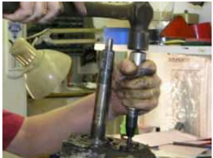
The countershaft can now be pushed out the back of the transmission with a rod. Once it is removed the countershaft gear cluster will fall to the bottom of the case.
