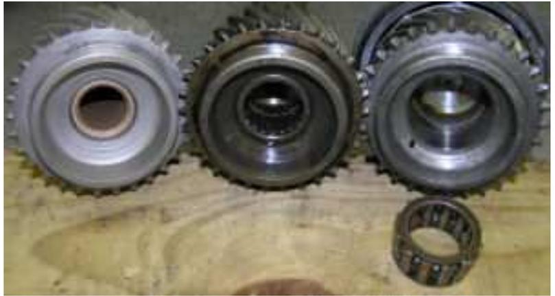
substituted for the bushing. The OD and ID for the cage bearing is 1.209 and 0.833, so it requires a different main shaft and cannot be directly substituted. Close ratio gearsets are designed for the cage type bearing, but come with a sleeve to adapt it for use with a shell type bearing and earlier main shaft.
