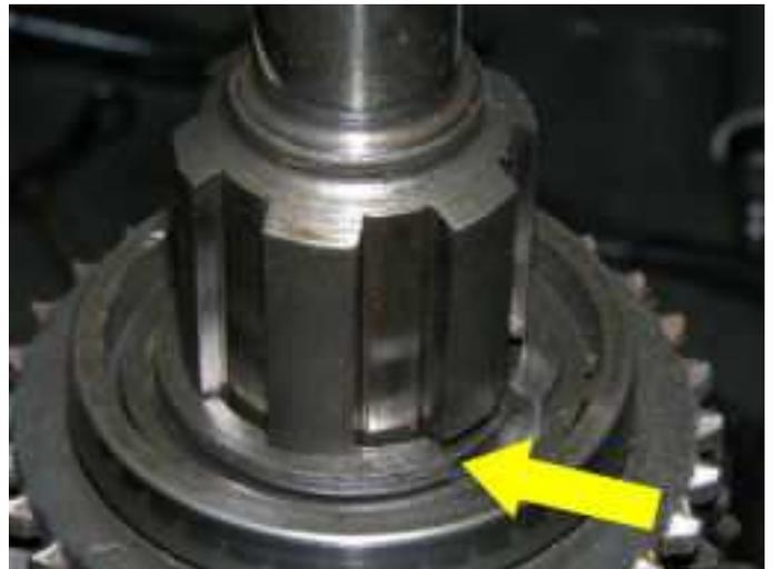
Once the clip is removed, the two gears, two washers and two bushings can be removed from the shaft.
