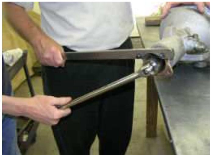
If you have an impact wrench, you can usually just hold the flange with your hand while you remove the nut. If you use an ordinary wrench, you'll probably need some sort of flange holding tool. Sam had this nice tool made, but you could also make one by drilling two holes in a piece of angle iron. Once the nut and washer are removed, you can tap the flange off with a small
