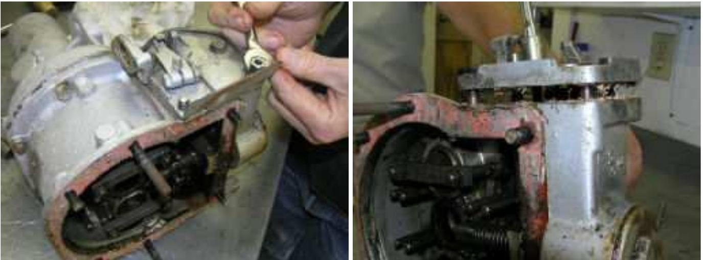
Once the plate is off and the springs withdrawn, the piston can be removed. Air pressure can be used to move the piston. Temporarily reinstall the ball in the operating valve, then (see photo) apply pressure at the operating valve plug hole. This initial movement can help to dislodge a stubborn piston. Sometimes air pressure will blow it completely out, so use a towel to catch it. You can now remove the operating valve.
