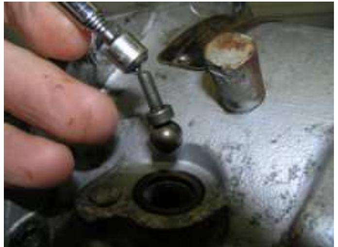
You can check the operation of the unit by reinstalling the ball, applying air pressure at the plug hole and manually activating the operating valve. The operating pistons should move the sliding assembly forward until the brake ring is contacted.
