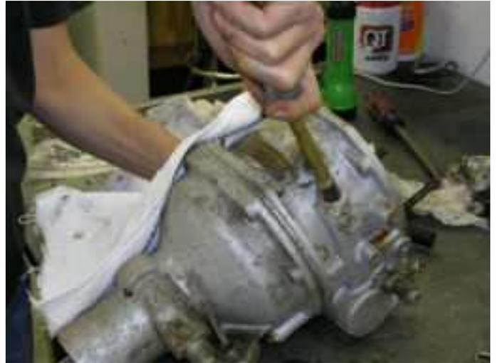
The early overdrives (models 22/1374 and 22/1712) have a large accumulator and piston. The piston has threads that are 3/8x24 so it can be removed by prying on the head of a long bolt screwed into the piston.
