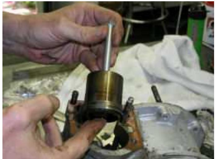
The later overdrives (models 22/1753 and 22/1985) with small accumulator have a sleeve and spacer tube in addition to the piston. If air pressure does not remove all three pieces, you can make an extraction tool using a rubber expansion plug (like a drain plug for a boat). A good hardware store will stock rubber expansion plugs in a variety of sizes.
